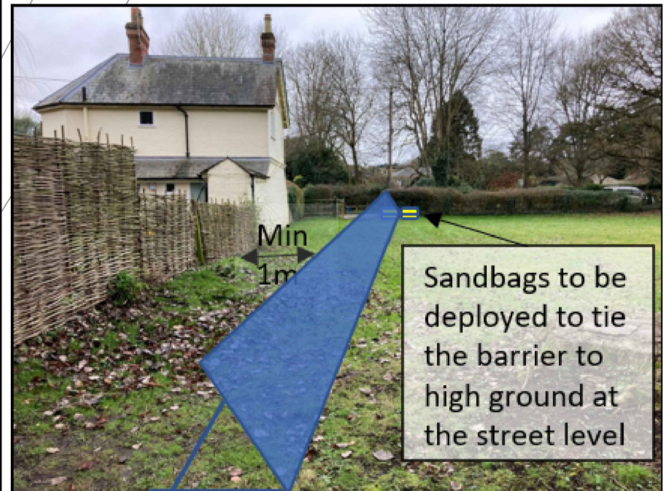
PHOTO A: BARRIER PARALLEL TO SPRINGHILL LODGE WITH 1m MAINTENANCE CORRIDOR ON THE DRY SIDE OF THE BARRIER
